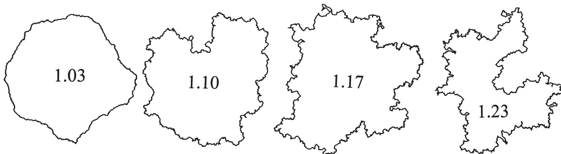
Fig. 8. Illustration of the visual appearance of the roughness of boundaries of fractal objects showing fractal dimensions between 1.00 and 1.23 (after Russ [9]).
