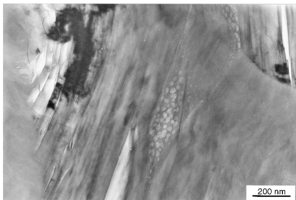
Fig. 2. Clusters of cavities in a graphite grain in SiC/C observed before implantation.
